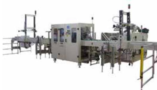
PRINTER IN LINE: DHDT for PAILS/TUBES systems
